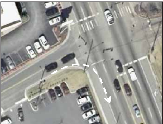
Most intersections on Broadway have large curb radii; the paved shoulder makes them effectively larger.
