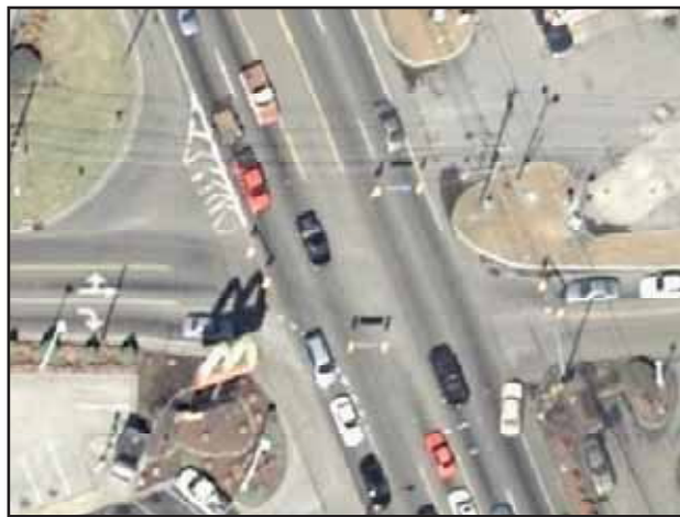
Most intersections on Broadway have large curb radii; the paved shoulder makes them effectively larger.
