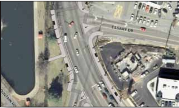
Cedar to Essary: Proposed intersection improvements for Cedar Drive and Essary Drive include sidewalks, crosswalks/pedestrian indications and raised right turn islands with pedestrian refuges. The construction of a right turn island at Essary Drive will require that southbound left turns be prohibited.
