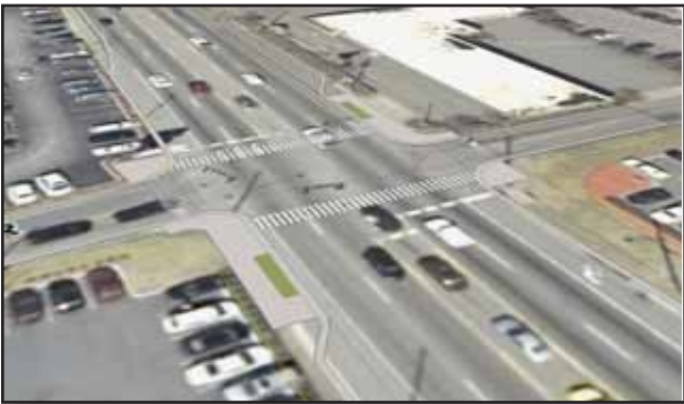
Broadway and Woodrow Drive: Proposed intersection improvements include reduced curb radii, curb extensions and ramps and transit pads.
