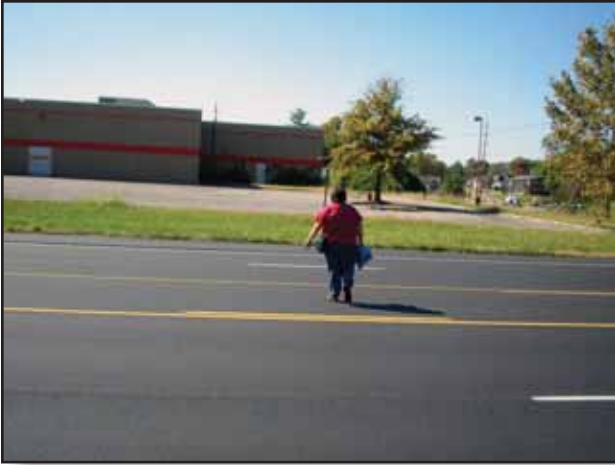
The lack of good, frequent crossing opportunities for pedestrians on Broadway is evident in the number of mid-block crossings in the flush median.
