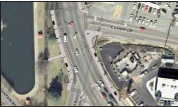
Cedar to Essary: A second option for Essary Drive is to replace the right turn island with a curb extension. Southbound left turns are permitted, but northbound right turns are not.
