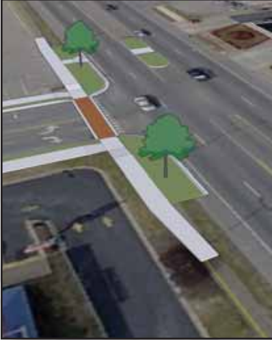
Aligning curb extensions with raised median islands is an effective, low-cost strategy for creating safe crossing opportunities.
